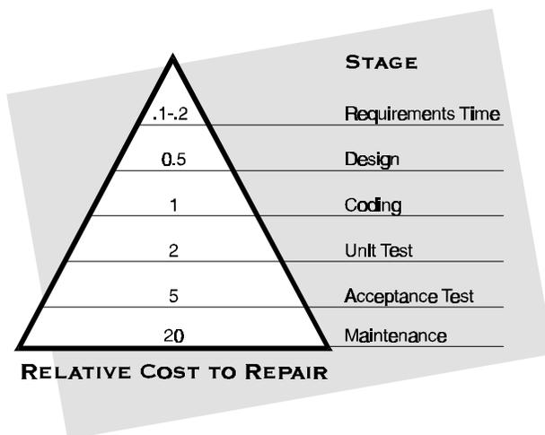
*Figure 1- As much as a 200:1 cost savings results from finding errors in the requirements stage versus finding errors in the maintenance stage of the software life-cycle.*
